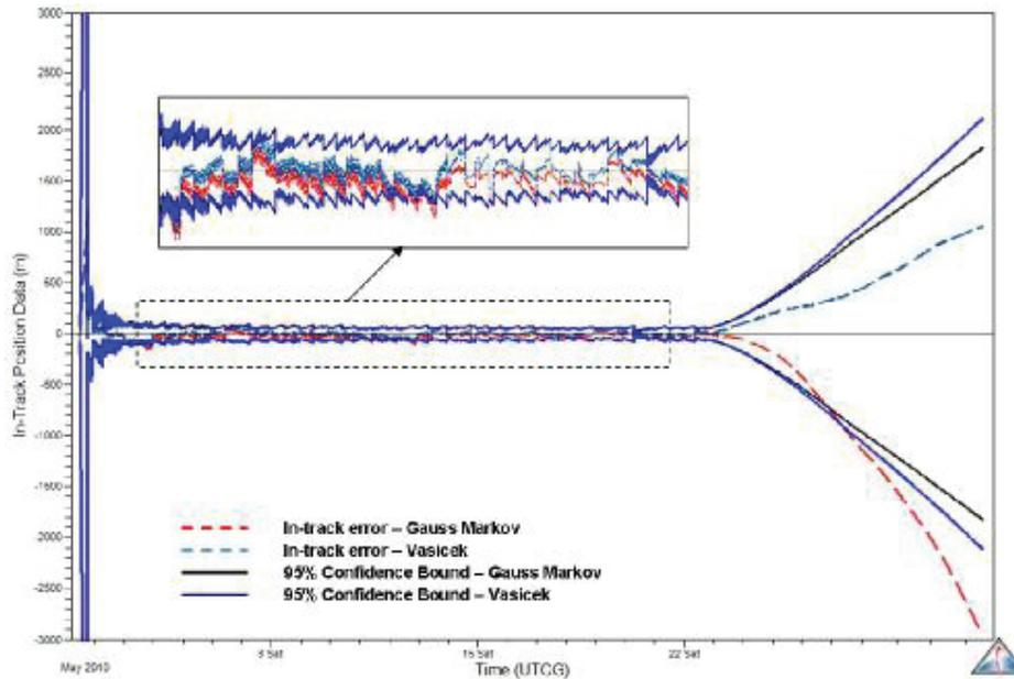
Figure 9. Propagation of *Gauss-Markov* and *Vasicek* Estimates.
