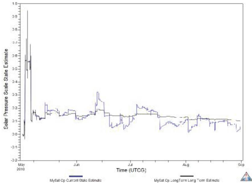
**Figure 7. 10% Positively Biased Solar Pressure Scale, 7-Day Half-Life, +10.6%**
