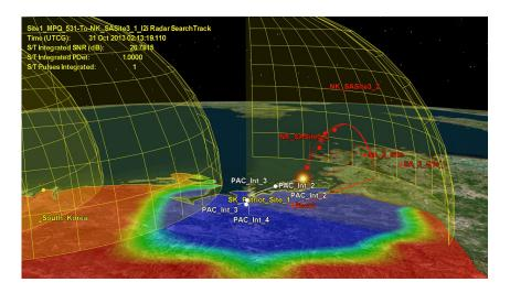
contours and beam volumes for antenna gain patterns and RCS patterns in STK's 2D and 3D graphics windows. *Radar* also works with STK's *Coverage* and *Analysis Workbench* to compute and display jamming and interference analyses on planar coverage grids and spatial volume grids, respectively.
