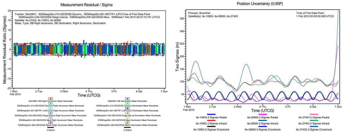
**Figure 9. Residual Ratios and Smoother Position Uncertainty LEO SBSS and SSN trackers and GEO RSO satellites.** These plots show the residual ratios and the position uncertainties for the SBSS scenario. The RSO state is derived from an IOD process and then a short LS run.
