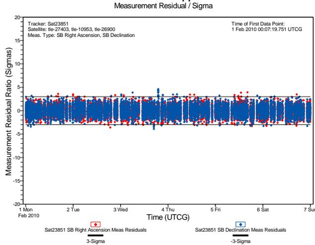
**Figure 4. Filter Residual Ratios LEO SBSS tracker and GEO RSO satellites.** This plot shows the residual ratios for the SBSS scenario. This case has the exact initial satellite state vectors from simulated data with all errors turned on. There are 3 satellites in the filter model here.
