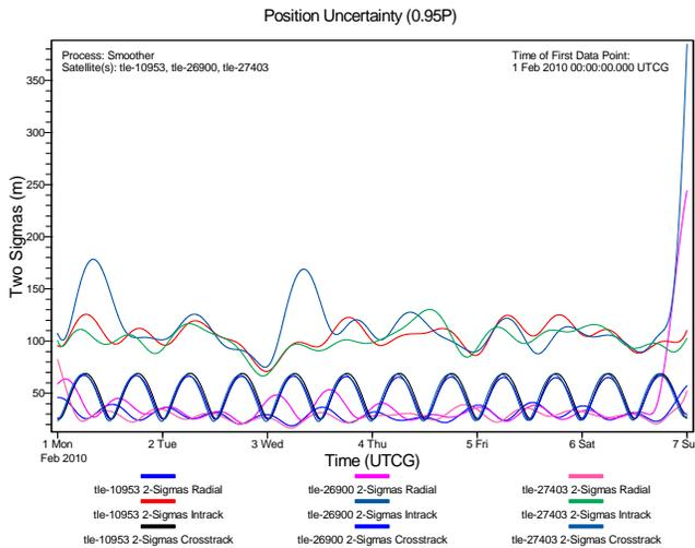
**Figure 5. Smoother Position Uncertainty LEO SBSS tracker and GEO RSO satellite.** This plot shows the smoother position uncertainty for the SBSS scenario. This case has the exact initial satellite state vectors from simulated data with all errors turned on. There are 3 satellites in the filter model here.
