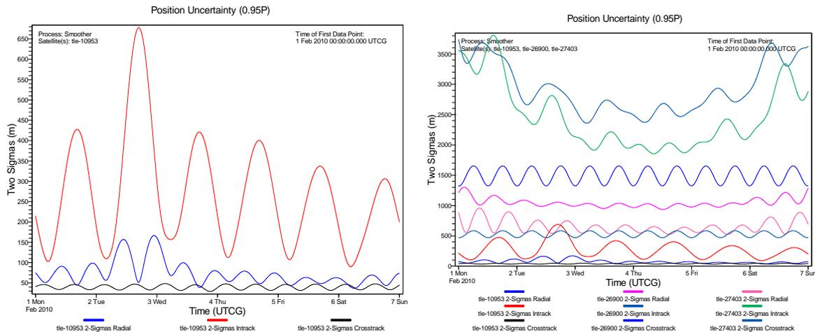
**Figure 11. Smoother Position Uncertainty GEO SBSS tracker and GEO RSO satellites.** The left hand plot shows the results for processing the single RSO satellite. The right hand plot shows the results when processing 3 RSO satellites. The initial satellite 10953, is the same in both plots. All RSO states are derived from an IOD process.
