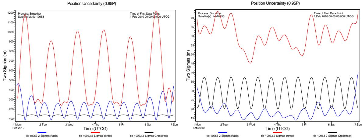
**Figure 10. Smoother Position Uncertainty LEO SBSS tracker and GEO RSO satellite.** The left hand plot shows the results for processing the single RSO satellite. The right hand plot shows the results when processing 5 RSO satellites. Notice the improvement in the multiple satellite solution. All RSO states are derived from an IOD process.
