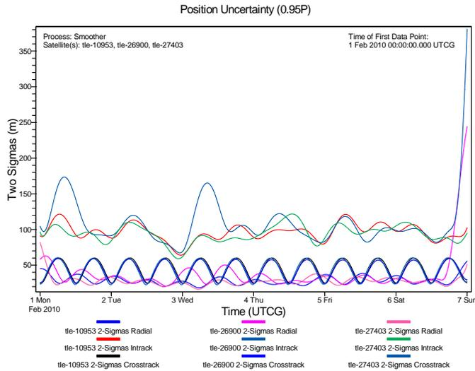
**Figure 7. Smoother Position Uncertainty LEO SBSS tracker, GEO RSO satellite, and SSN.** This plot shows the position uncertainties for the SBSS scenario. This case has the exact initial satellite state vectors from simulated data with all errors turned on. There are 3 satellites in the filter model here.
