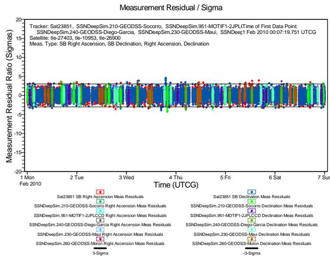
**Figure 6. Filter Residual Ratios LEO SBSS tracker, GEO RSO satellites, and SSN.** This plot shows the residual ratios for the SBSS scenario. This case has the exact initial satellite state vectors from simulated data with all errors turned on. There are 3 satellites modeled here and sensor observations from multiple SSN sites.
