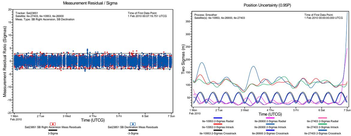
**Figure 8. Residual Ratios and Smoother Position Uncertainty LEO SBSS tracker and GEO RSO satellites.** These plots show the residual ratios and the position uncertainties for the SBSS scenario. The RSO state is derived from an IOD process and then a short LS run.
