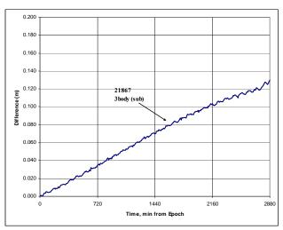
Figure 18: Special-K Third-body Comparisons to STK/HPOP: Positional differences for a single satellite are shown. Note that these results are obtained by subtracting two runs in which only third body perturbations were different.
