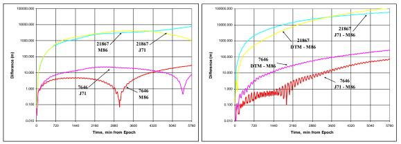
**Figure 22: GEODYN Ephemeris Comparisons to STK/HPOP:** Results are given for Starlette (07646) and JERS (21867). The left plot shows the comparisons while the right plot shows the difference from simply switching atmospheric models. The scales are the same. Note the comparison differences are smaller than the differences resulting from simply changing the atmospheric model.
