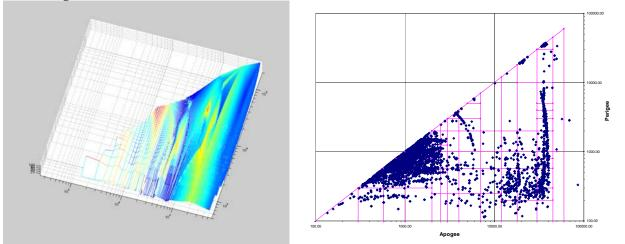
**Figure 1 : Visualizing the Space Catalog:** This figure shows two perspectives for the space satellite catalog. The left plot shows apogee vs perigee values, with inclination being the vertical axis. Note that the red color indicates higher inclination values. The dark blue orbits are generally below about 30 degrees inclination. The right plot shows the traditional two-dimensional apogee – perigee relations. Between the two, you can estimate the number of satellites in a particular region.
