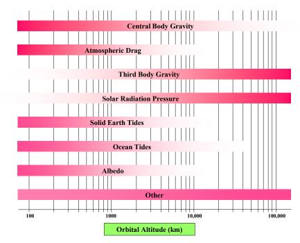
**Figure 2 :** Generic Force Model Setup: This figure shows approximate force model setups for various orbital altitudes. Note that specific accuracy requirements may extend the areas of applicability, and hence the faded color bars. Additionally, the eccentricity will also require additional force models not depicted here.
