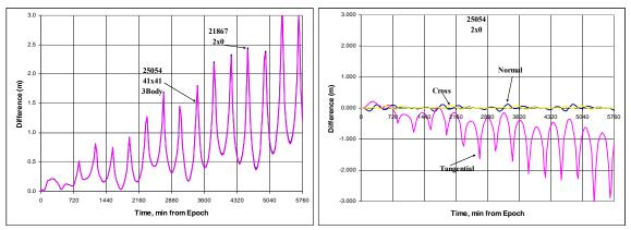
**Figure 15 : GTDS Regularized Time Gravitational Comparisons to STK/HPOP:** Data is shown for 25054 using regularized time for two force model combinations including NTW differences. Note the differences are somewhat larger than the previous examples, but still more than an order-of-magnitude less than the effect of simply truncating from  $70 \times 70$  to a  $60 \times 60$  field.
