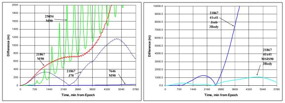
Figure 20: TRACE and GTDS Atmospheric Drag Comparisons to STK/HPOP: Several satellites are shown using the MSIS-90 and Jacchia-Roberts atmospheric models.
