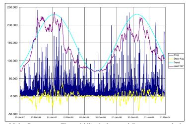
**Figure 9:** Variability of Solar Parameters: The variability in the  $a_p$  and  $F_{10.7}$  parameters is shown for about the last two solar cycles. Note that the  $a_p$  difference ("D ap", daily vs the maximum 3 hourly value) is almost as large as the measurements themselves. Also note the  $F_{10.7}$  difference ("Dlast – Avg", centered vs. last 81-days) can be 30-50 solar flux units.
