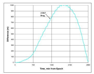
Figure 21: Special-K Atmospheric Drag Comparisons to STK/HPOP: A single test for atmospheric drag was conducted by comparing two runs in which only atmospheric drag was different.
