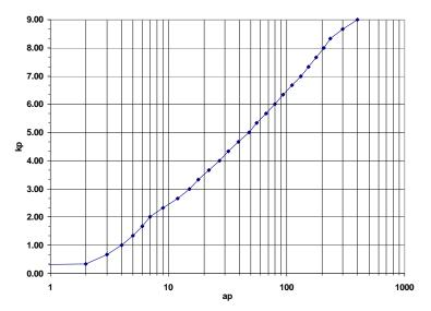
Figure 10: Relationship between  $a_p$  and  $K_p$ : The semi-logarithmic correlation between  $a_p$  and  $K_p$  is shown. Note that there are only distinct values that correspond between each scale and  $K_p$  is multiplied by 10.0.
