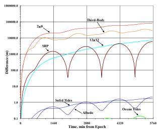
**Figure 7:** Force Model Comparisons – GEO 35786×35790 km, 0.0°: This figure shows RSS position differences for a simplified numerical propagator and force model truncation. This is the Galaxy 11 satellite, SSC# 26038.
