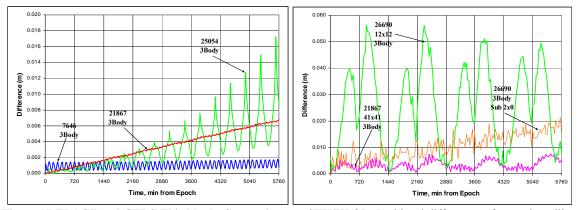
Figure 17:TRACE and GTDS Third-body Comparisons to STK/HPOP: Positional differences of several satellites are shown for third-body forces. The "sub" line in the GTDS graph represents the difference of runs of combined forces to better show the effect of just third-body forces. The higher line contains the original signature from the gravitational forces.
