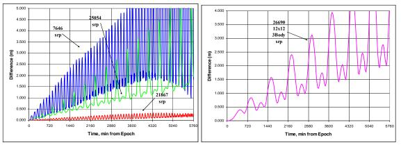
Figure 19: TRACE and GTDS Solar Radiation Pressure Modeling Comparisons to STK/HPOP: Several satellite positional differences are shown for solar radiation pressure. Although the results show meter-level differences, these are orders of magnitude below the effects of the dominant other forces.
