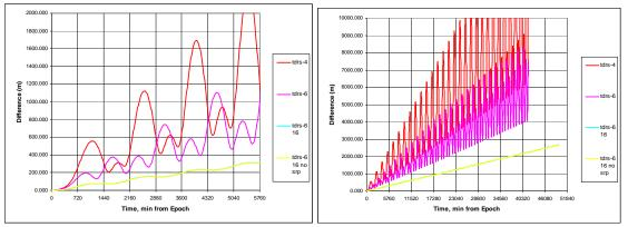
**Figure 24: GEODYN Ephemeris Comparisons to STK/HPOP :** Results are given for TDRS-4 and TDRS-6. The scales are different to show 4-day and ~30-day performance. The differences show the importance of obtaining a good initial state.
