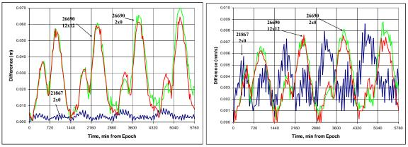
**Figure 13: GTDS Gravitational Comparisons to STK/HPOP:** Two satellites are shown with varying gravity field sizes. The positional differences are on the left and the velocity differences are on the right. Note that similar shapes between the two plots and that all the results are less than 0.07 m (0.009 mm/s) after 4 days of propagation.
