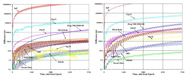
**Figure 4 :** Force Model Comparisons – LEO 800×1100 km, 49.8° and LEO 550×3020 km, 32.8°: This figure shows RSS position differences for a simplified numerical propagator and force model truncation. This is the Starlette, SSC# 7646 and Vanguard II, SSC# 11.
