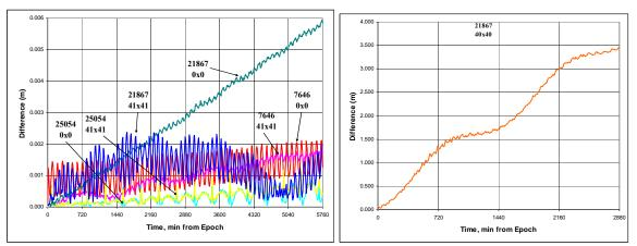
**Figure 16:TRACE and Special-K Gravitational Comparisons to STK/HPOP:** Three satellites are shown with various gravity fields for TRACE. Note the close comparisons for all cases (< 1 cm) in 4 days. The Special-K run for satellite 21867 showed a slight drift over 2 days. This was not examined extensively but is probably a gravitational constant or integrator issue.
