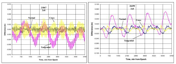
Figure 14: GTDS Component Differences to STK/HPOP: NTW components are given for the  $2\times0$  21867 case, and the  $2\times0$  26690 case. Note that the primary effect is along-track – aligned with the velocity vector direction. A signature appears with the GPS (26690) propagation that was not resolved.
