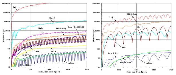
**Figure 5:** Force Model Comparisons – LEO 1300×1300 km, 66° and MEO 20000×20000 km, 55.2°: This figure shows RSS position differences for a simplified numerical propagator and force model truncation. This is the TOPEX, SSC# 22076 satellites, and the GPS, SSC# 26690 satellites.
