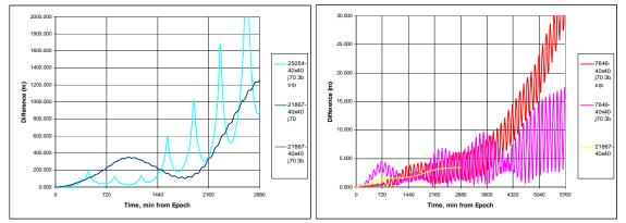
**Figure 23: Special-K Ephemeris Comparisons to STK/HPOP:** Results are given for several satellites. Notice that the scales are not the same. Also recognize the drifting signature present in all the comparisons. The 21867 40x40 gravity field case is shown to highlight the "signature".
