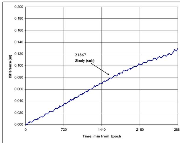
**Figure 18: Special-K Third-body Comparisons to STK/HPOP:** Positional differences for a single satellite are shown. Note that these results are obtained by subtracting two runs in which only third body perturbations were different.
