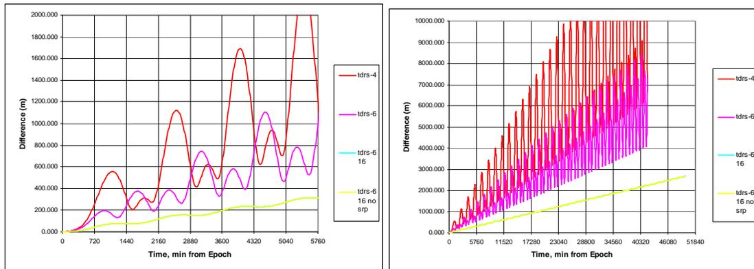
**Figure 24: GEODYN Ephemeris Comparisons to STK/HPOP :** Results are given for TDRS-4 and TDRS-6. The scales are different to show 4-day and ~30-day performance. The differences show the importance of obtaining a good initial state.
