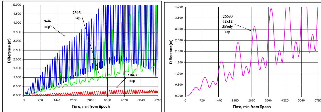
**Figure 19: TRACE and GTDS Solar Radiation Pressure Modeling Comparisons to STK/HPOP:** Several satellite positional differences are shown for solar radiation pressure. Although the results show meter-level differences, these are orders of magnitude below the effects of the dominant other forces.
