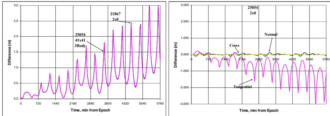
**Figure 15 : GTDS Regularized Time Gravitational Comparisons to STK/HPOP:** Data is shown for 25054 using regularized time for two force model combinations including NTW differences. Note the differences are somewhat larger than the previous examples, but still more than an order-of-magnitude less than the effect of simply truncating from 70x70 to a 60x60 field.
