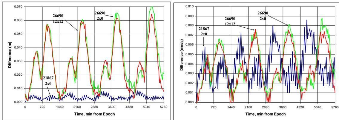
**Figure 13: GTDS Gravitational Comparisons to STK/HPOP:** Two satellites are shown with varying gravity field sizes. The positional differences are on the left and the velocity differences are on the right. Note that similar shapes between the two plots and that all the results are less than 0.07 m (0.009 mm/s) after 4 days of propagation.
