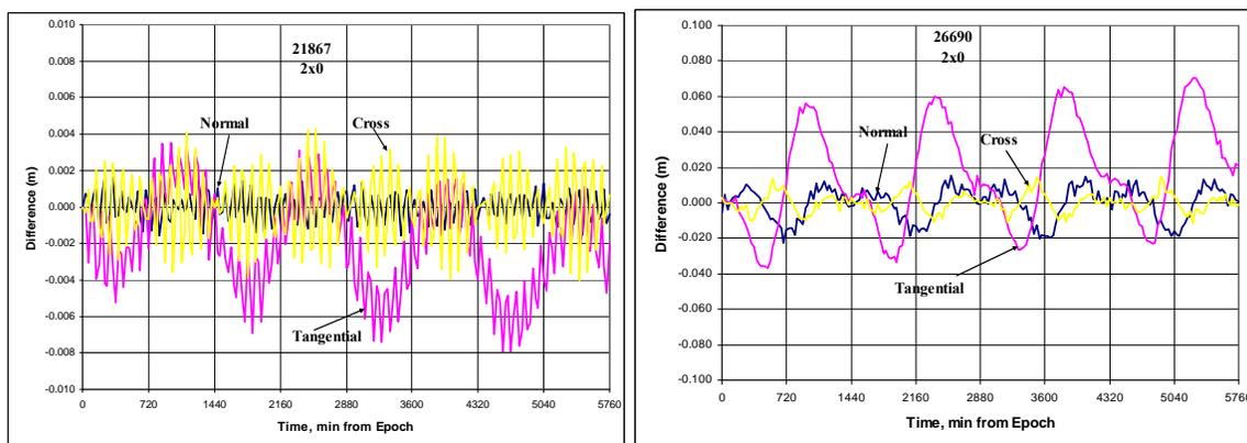
**Figure 14: GTDS Component Differences to STK/HPOP:** NTW components are given for the 2x0 21867 case, and the 2x0 26690 case. Note that the primary effect is along-track – aligned with the velocity vector direction. A signature appears with the GPS (26690) propagation that was not resolved.
