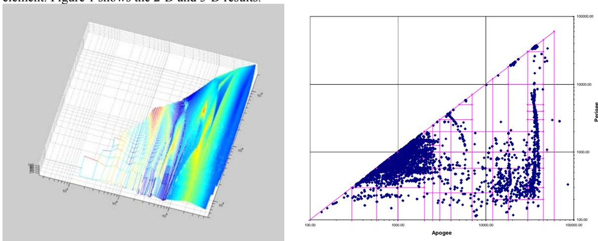
**Figure 1 : Visualizing the Space Catalog:** This figure shows two perspectives for the space satellite catalog. The left plot shows apogee vs perigee values, with inclination being the vertical axis. Note that the red color indicates higher inclination values. The dark blue orbits are generally below about 30 degrees inclination. The right plot shows the traditional two-dimensional apogee – perigee relations. Between the two, you can estimate the number of satellites in a particular region.
