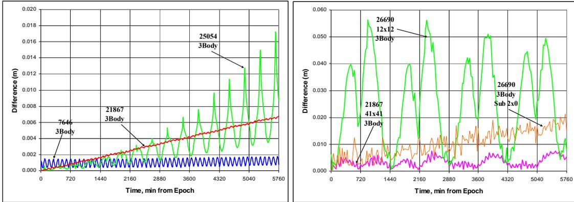
**Figure 17: TRACE and GTDS Third-body Comparisons to STK/HPOP:** Positional differences of several satellites are shown for third-body forces. The “sub” line in the GTDS graph represents the difference of runs of combined forces to better show the effect of just third-body forces. The higher line contains the original signature from the gravitational forces.
