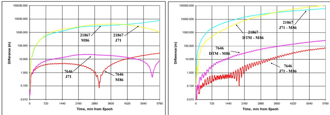
**Figure 22: GEODYN Ephemeris Comparisons to STK/HPOP:** Results are given for Starlette (07646) and JERS (21867). The left plot shows the comparisons while the right plot shows the difference from simply switching atmospheric models. The scales are the same. Note the comparison differences are smaller than the differences resulting from simply changing the atmospheric model.
