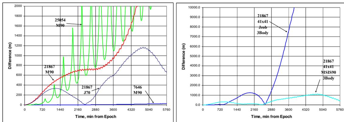
**Figure 20: TRACE and GTDS Atmospheric Drag Comparisons to STK/HPOP:** Several satellites are shown using the MSIS-90 and Jacchia-Roberts atmospheric models.
