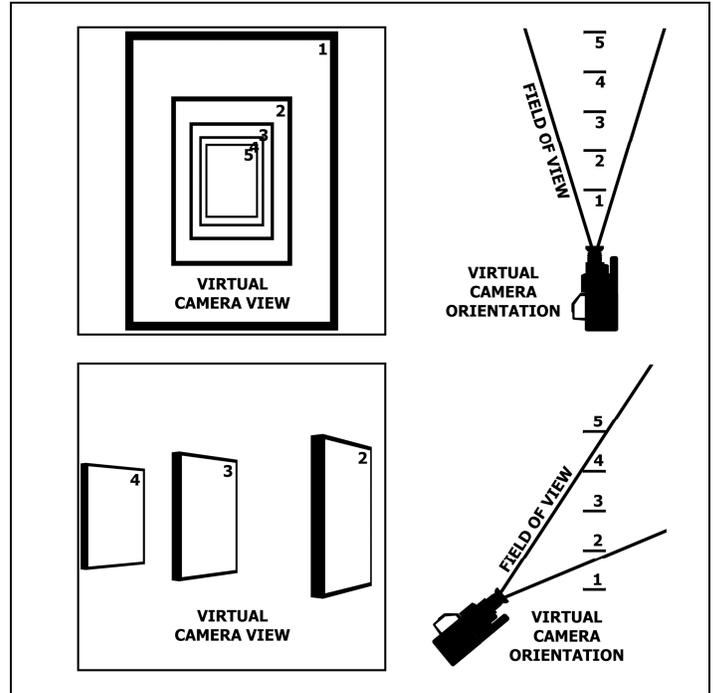
Figure 10: Virtual camera effect of viewing angle
