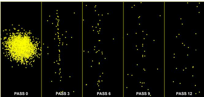
Figure 19: ECI based Radial debris dispersion with discrete markers used to represent the debris samples
