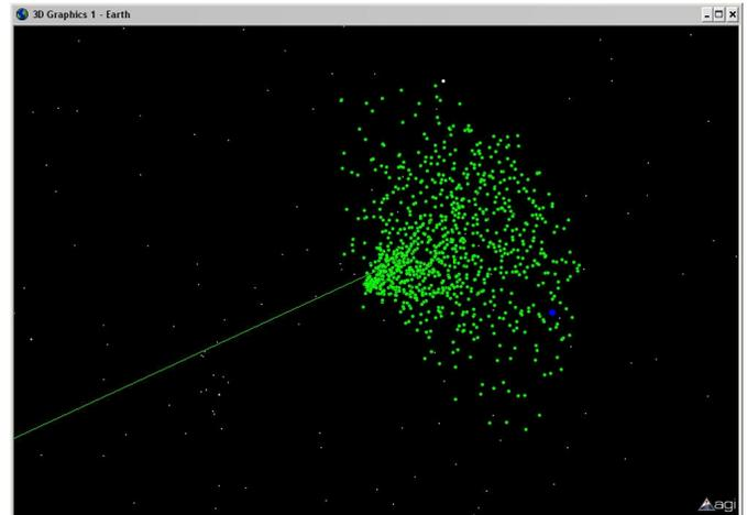
Figure 4: Generated Debris, Normal Distribution of  $\Delta V$
