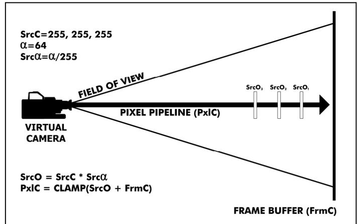
Figure 11: Pixel pipeline for debris environment
