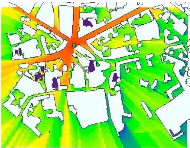
Figure 6. (U) Full 3D Path Loss, Milan, Italy
