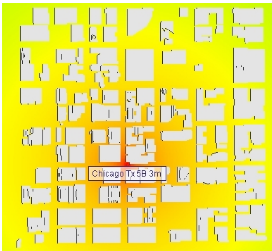
Figure 1. (U) Example of Hata statistical propagation loss calculated for Chicago, ignoring model limits.
