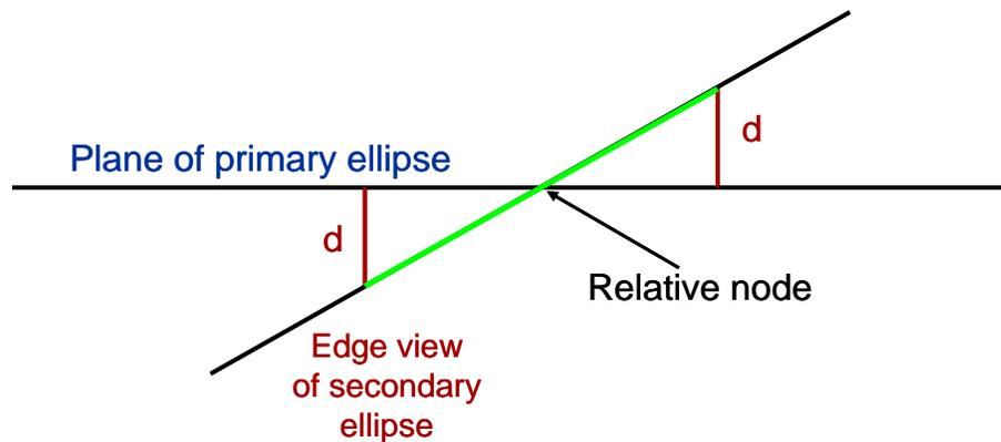
**Figure 5. Distance from Primary to orbit plane of Secondary<sup>9</sup>**
