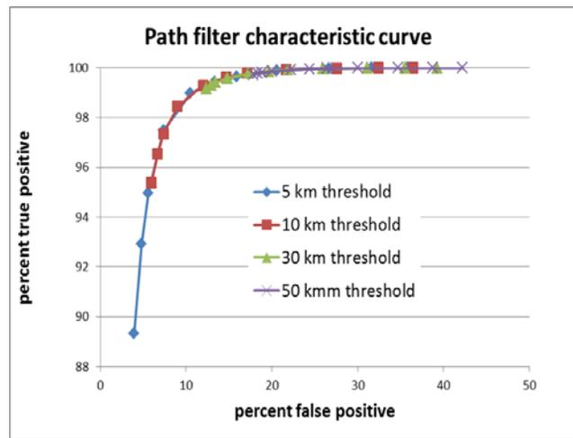
Figure 4c. Orbit-path filter true versus false positive rates
