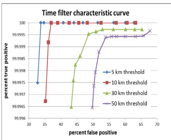
**Figure 8c. Time filter true versus false positive rates**
