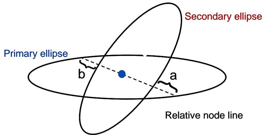
**Figure 3. Orbit Path Filter Principles<sup>9</sup>**
