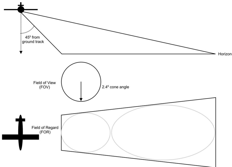
**Figure 2 –Aircraft sensor swath geometry**
