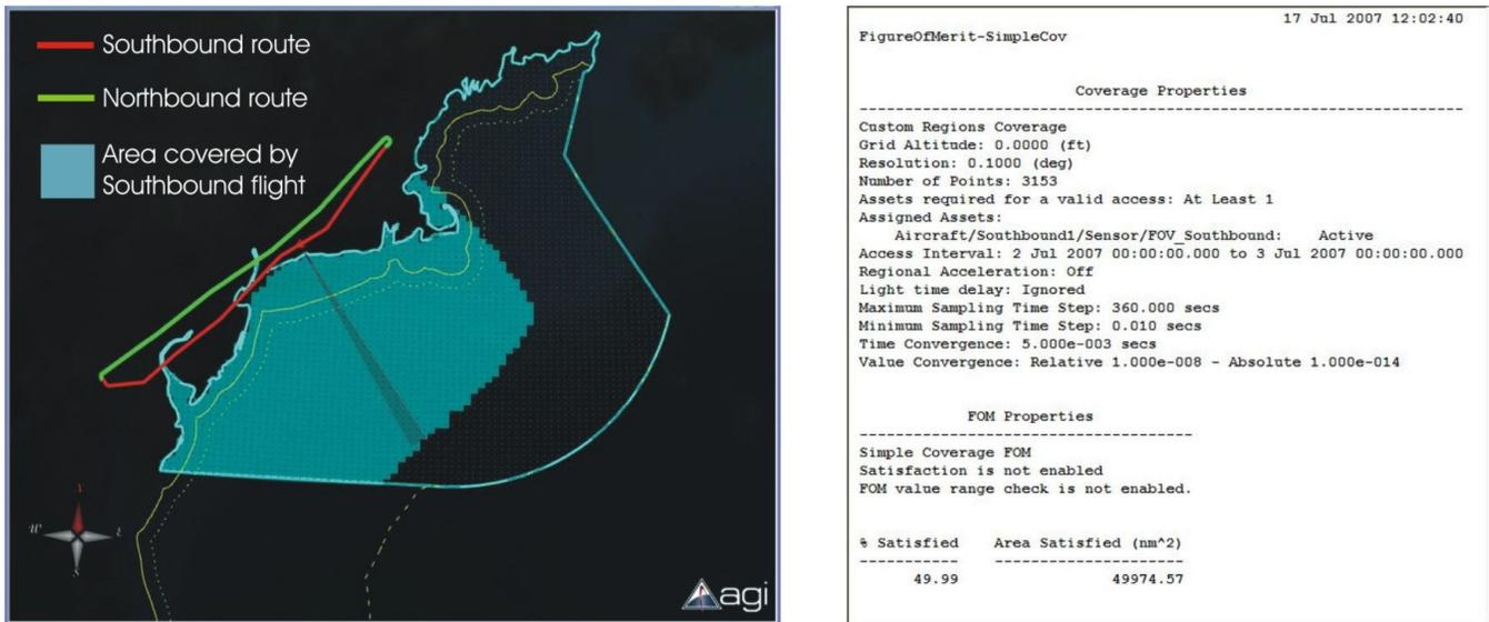
Figure 6 - Simple coverage, single aircraft southbound
