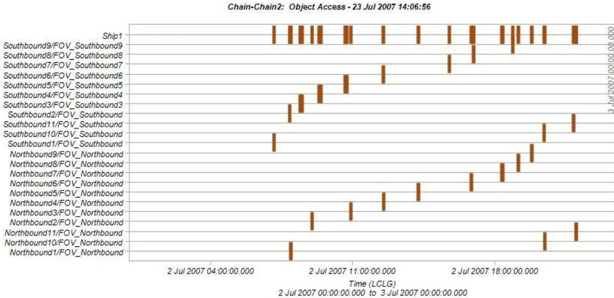
**Figure 14 –Times the sensors have access to the ship in 24 hours**
