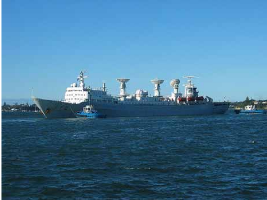
Figure 4: Chinese Space Surveillance Tracking Ship: Note the several large tracking dishes, similar to the Millstone Hill SSN tracking system. There are several other likely optical trackers, and since the ship designation is number 5, it is likely there are other ships with similar capabilities. Photo from Wikipedia (Yuanwang 2011)
