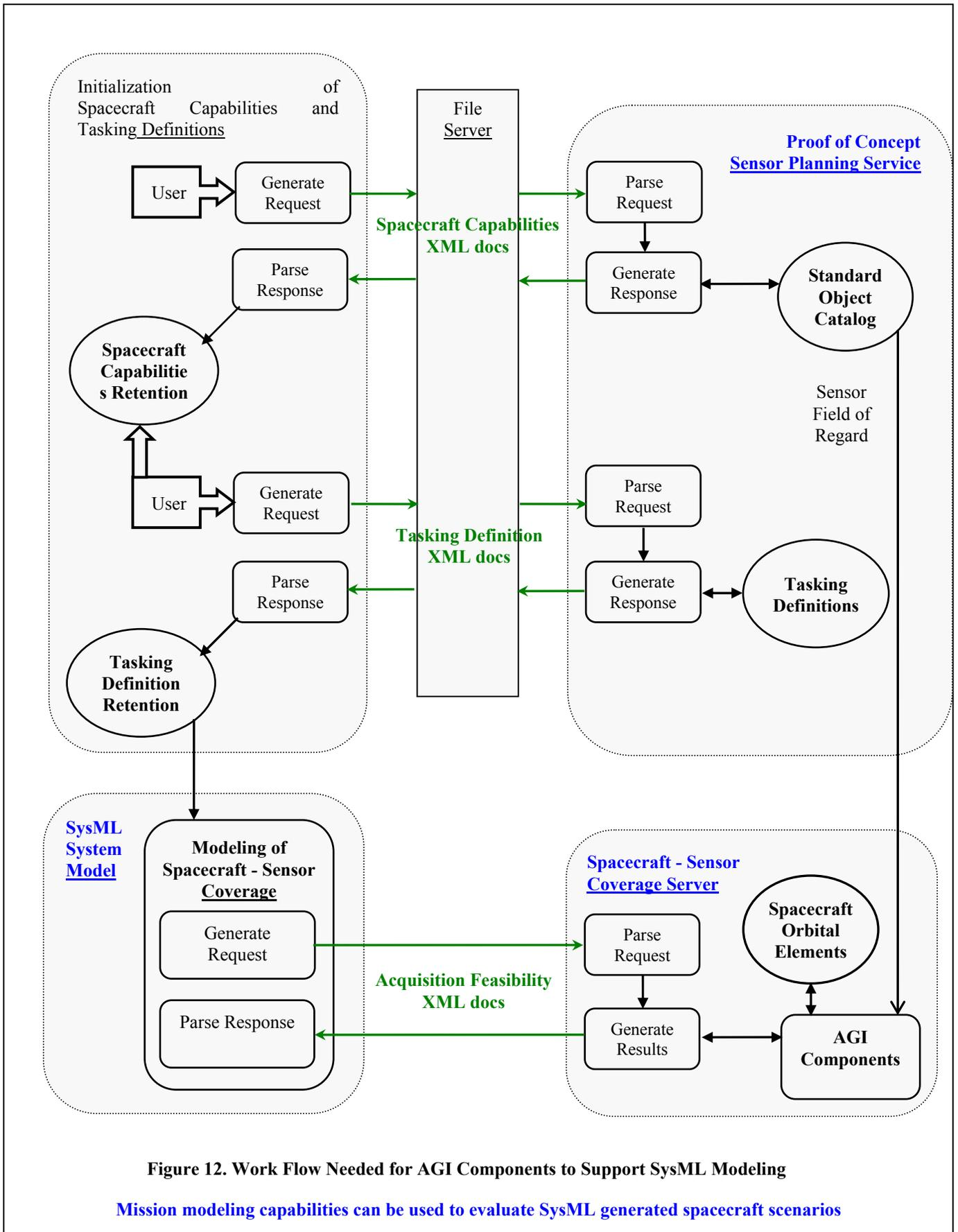
Figure 12. Work Flow Needed for AGI Components to Support SysML Modeling
