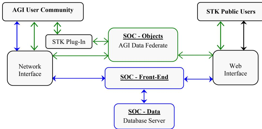
**Figure 9. Data Access - Standard Object Catalog**
