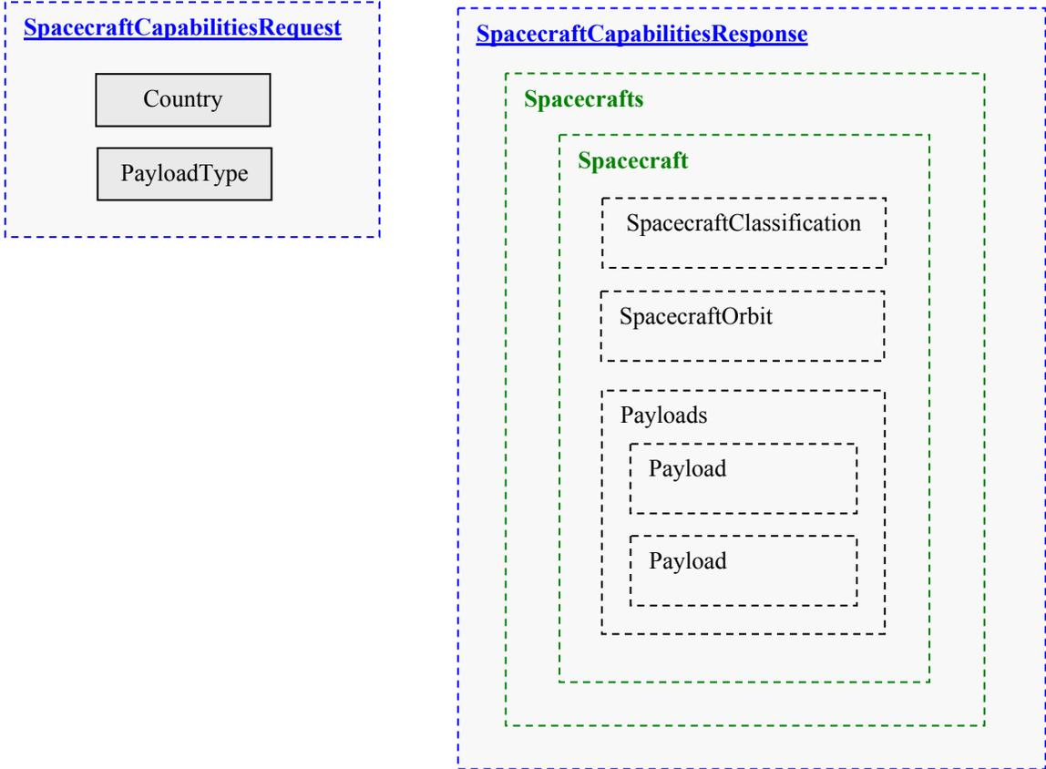
**Figure 5. Schema Overview of Prototype of Spacecraft Capabilities Request and Response XML Documents**
