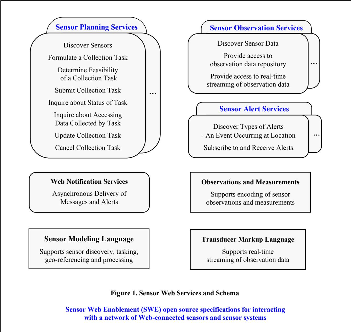
**Figure 1. Sensor Web Services and Schema**
