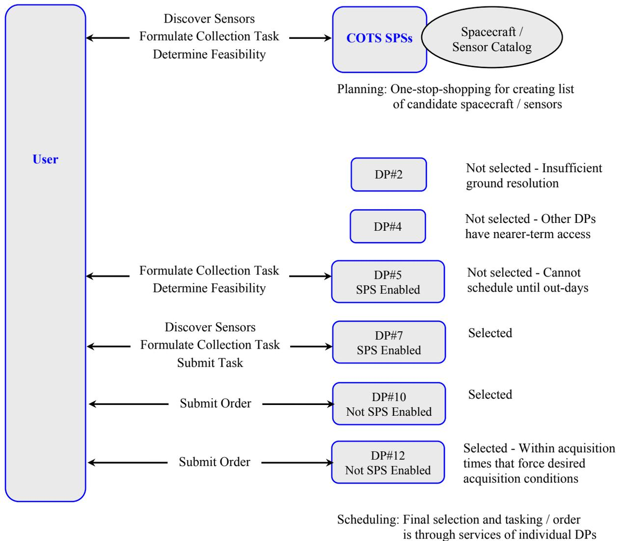
**Figure 3. Application of COTS GetFeasibility Operation**
