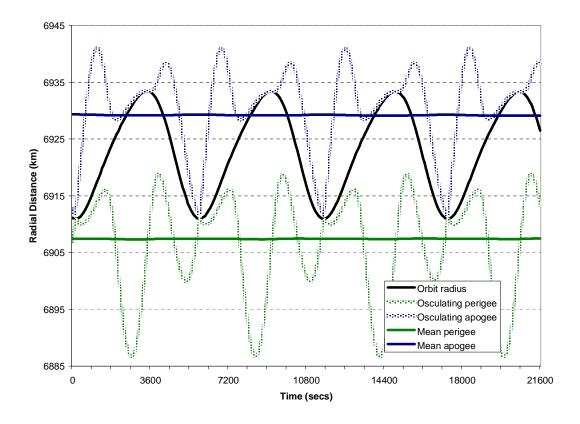
Figure 2. Comparison Of Computed Values Of Apogee And Perigee (LEO, SSC 26281)
