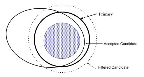
Figure 1. Apogee/Perigee Filter Geometry
