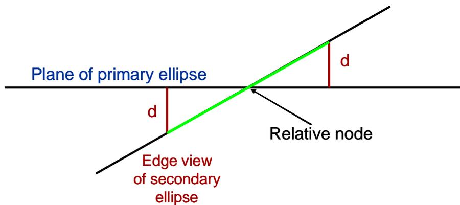
Figure 8. Distance From Primary To Orbit Plane Of Secondary
