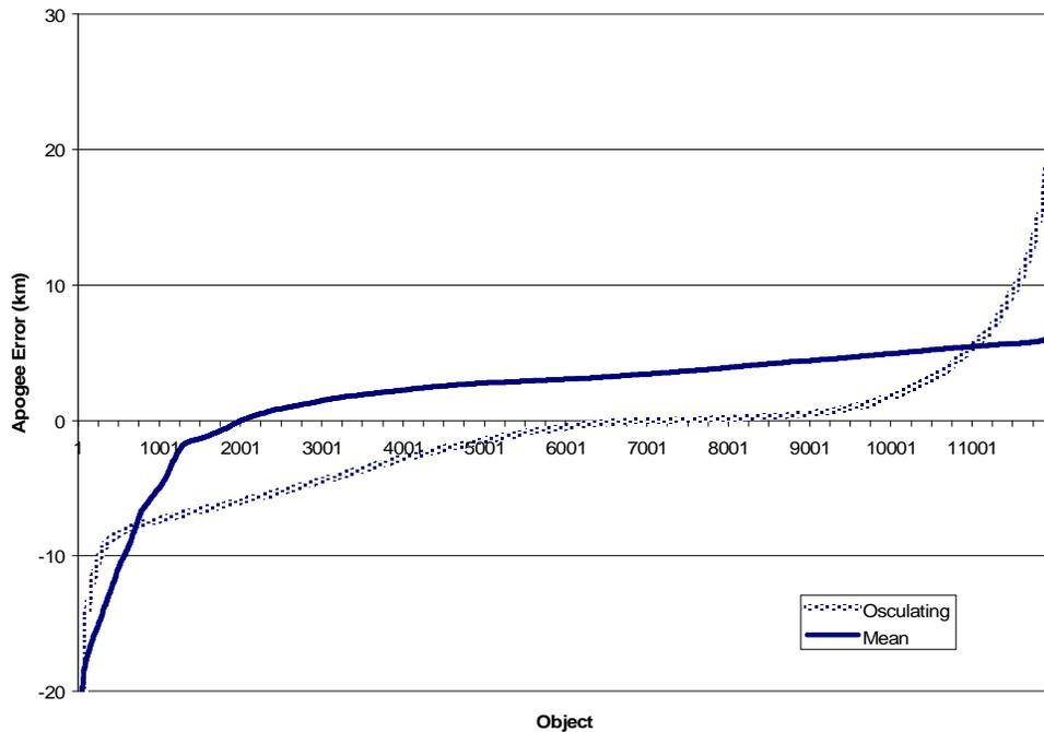
**Figure 5. Apogee Approximation Errors**
