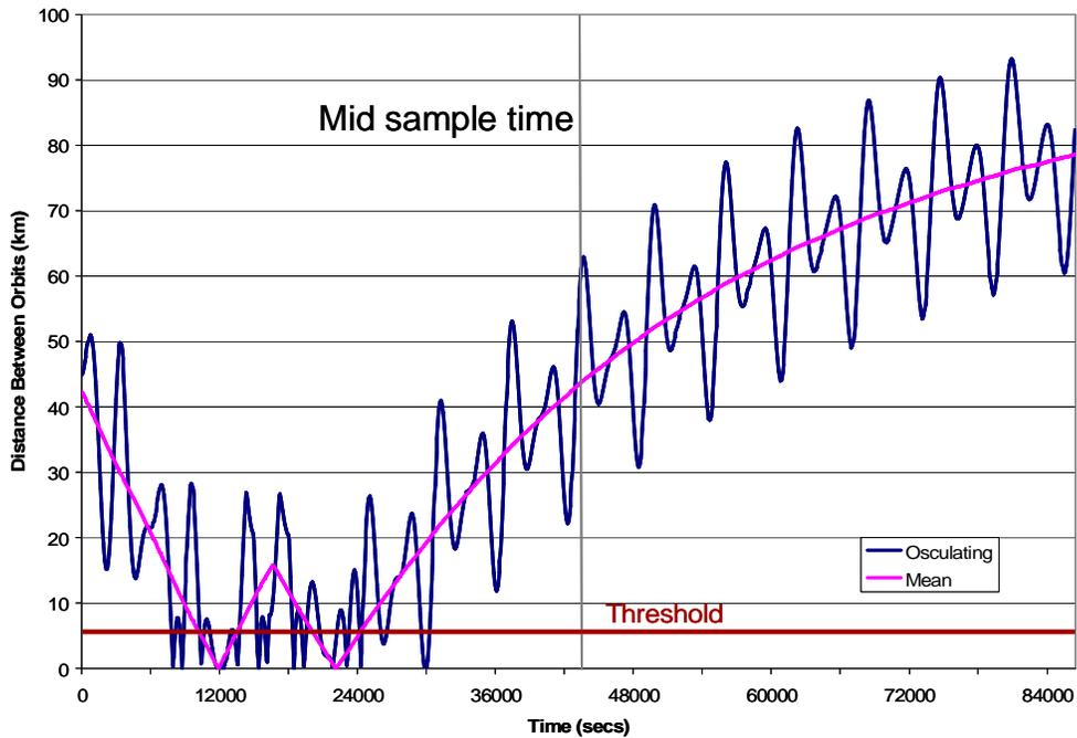
**Figure 7. Computed Distance Between Orbits Using Osculating And Mean Elements**
