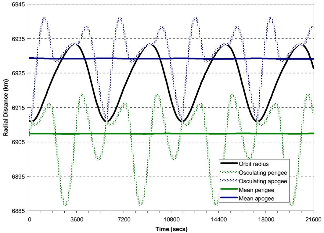
**Figure 2. Comparison Of Computed Values Of Apogee And Perigee (LEO, SSC 26281)**
