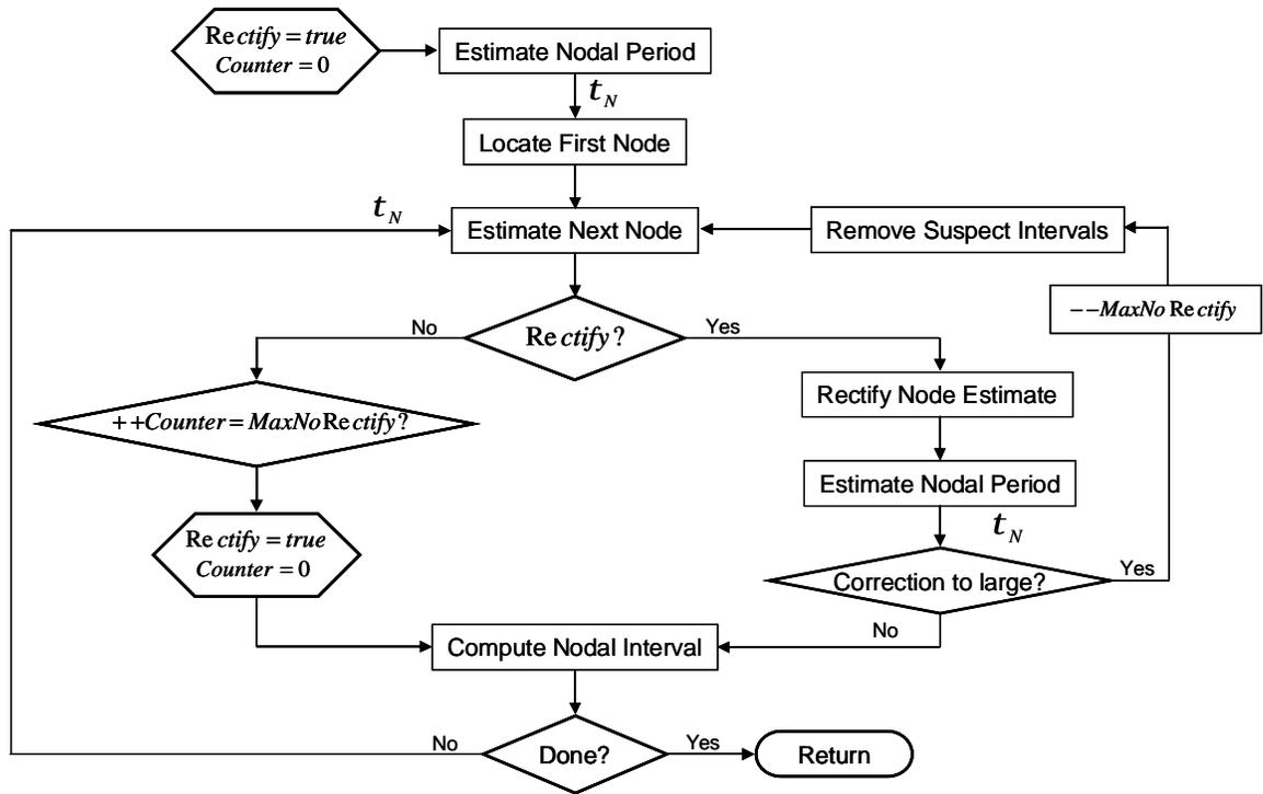
Figure 10. Relative Node Interval Generation
