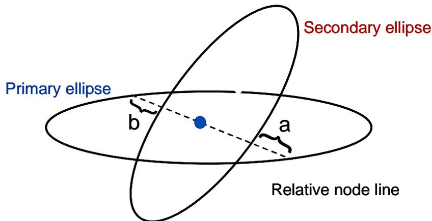
**Figure 6. Orbit Path Filter Geometry**
