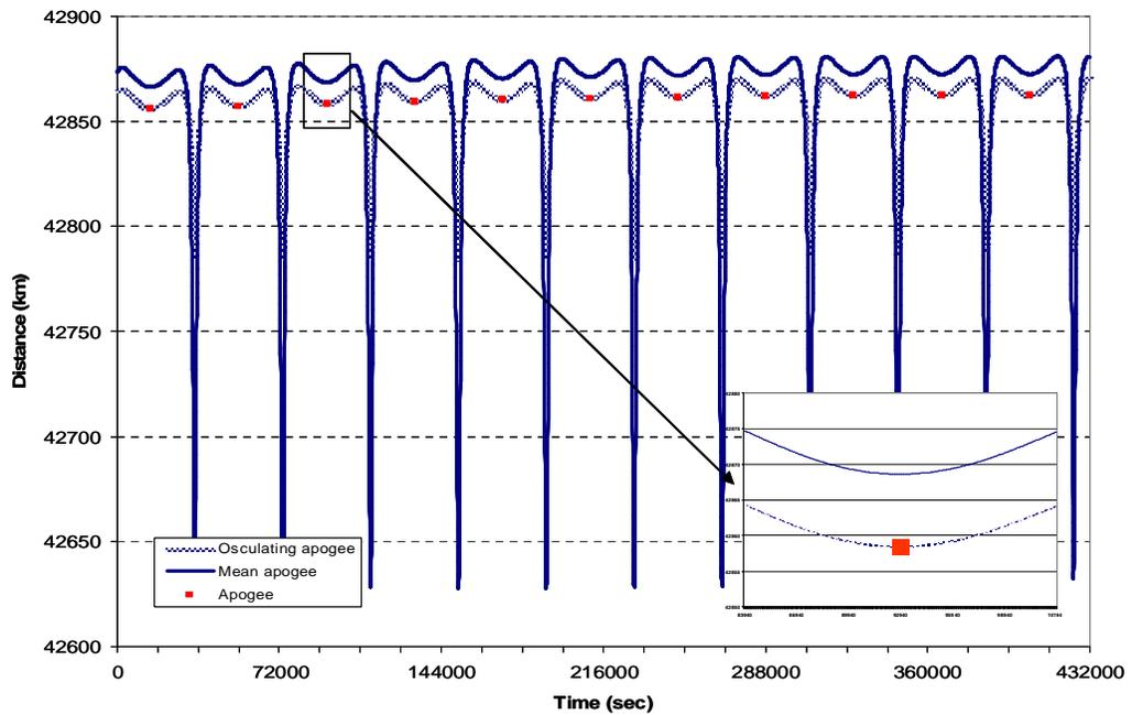
**Figure 3. Comparison Of Computed Values Of Apogee And Perigee (HEO, SSC 23687)**
