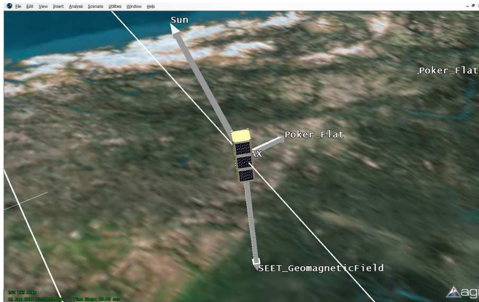
Figure 5. STK-generated schematic of RAX spacecraft with vectors pointing towards the experimental zone, Poker Flat, AK, the sun, and along the Earth’s magnetic field.
