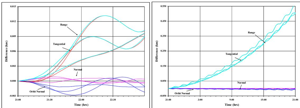
**Figure 5: ICESat POE Ephemeris Comparisons:** Results are given for ICESat at 2 hours (left) and at 1 day (right) using three different starting locations (each differs by 20 minutes). Notice the difference in the short term results.
