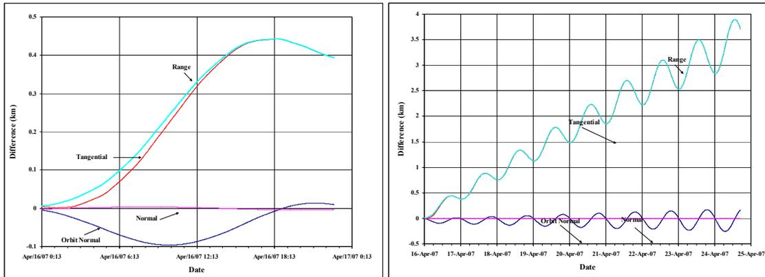
**Figure 16: GEO OD Ephemeris Comparisons:** Results are given for a GEO satellite after a 2 day OD of observational data. The difference after 1 day is about 400m.
