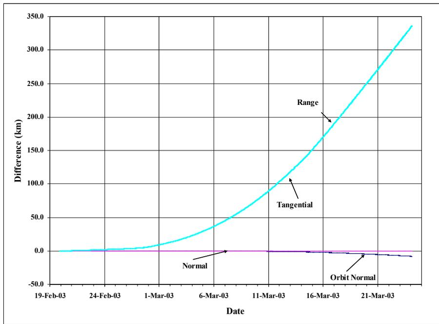
**Figure 4: ICESat POE Ephemeris Comparisons Including Maneuvers:** When the maneuvers are included, the performance is smoother, although not as good as it could be.
