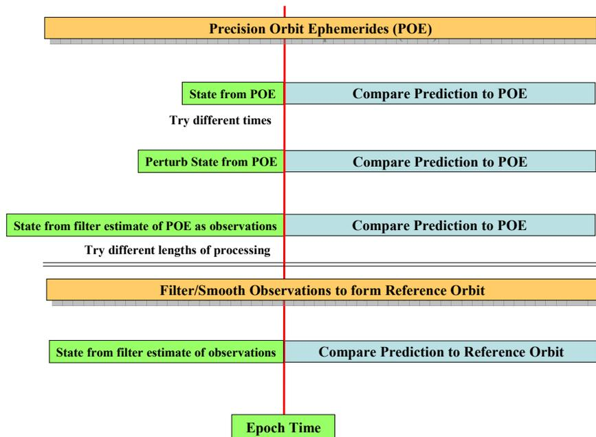
**Figure 1: General setup for Prediction Comparisons :** Several comparisons are found using the POE's directly. Other orbits require generation of reference orbits. The distinction is important as the independent nature and accuracy are not generally the same.
