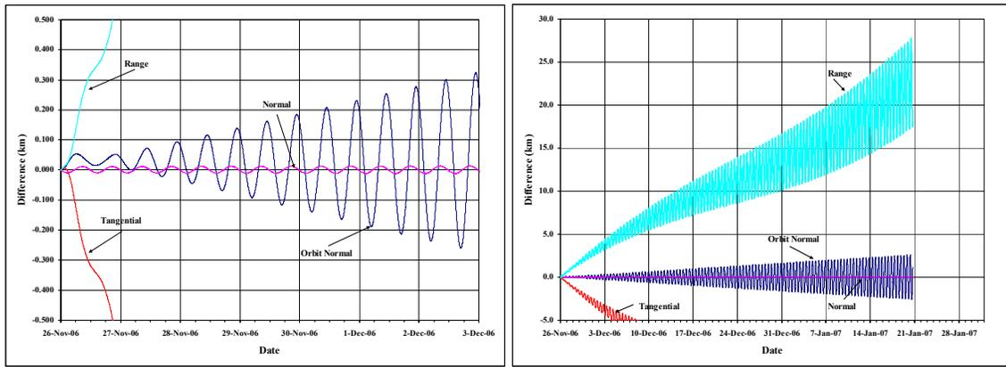
**Figure 10: GPS SVN-31 POE Ephemeris Comparisons:** Results are given for GPS SVN-31 at the four time intervals. The rapid departure suggests some of the modeling is not properly set.
