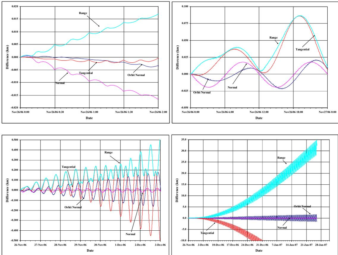
**Figure 9: GPS SVN-22 POE Ephemeris Comparisons:** Results are given for GPS SVN-22 at the four time intervals. Notice that the change in behavior at about the 2-3 week point.
