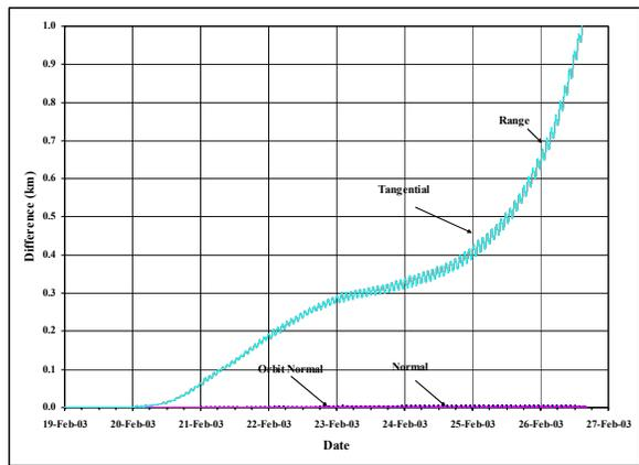
**Figure 13: ICESAT OD and POE Ephemeris Comparisons:** Results are given for ICESAT after a 1 day OD of the POE data. The tangential difference still dominates very quickly, but the overall results are much better than the original prediction because the satellite parameters are better known from the OD portion of the run.
