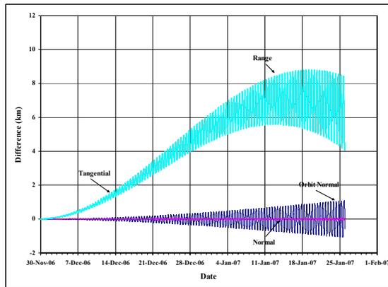
**Figure 15: GPS SVN-31 OD and POE Ephemeris Comparisons:** Results are given for GPS SVN-31 after a 4 day OD of the POE data. Notice the smoother overall performance of the differences and the significant improvement from Fig. 10.
