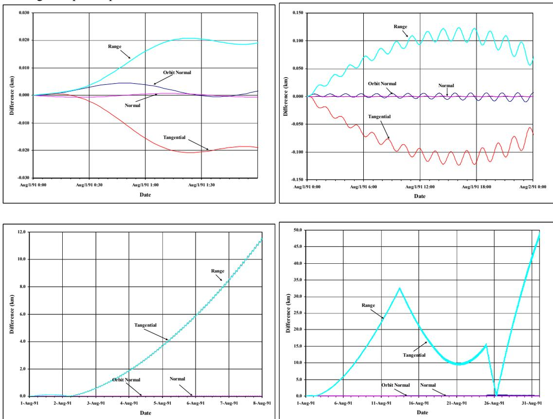
**Figure 6: ERS-1 POE Ephemeris Comparisons:** Results are given for ERS-1 at the four time intervals. Notice that the pronounced appearance of maneuvers in the long range comparison.
