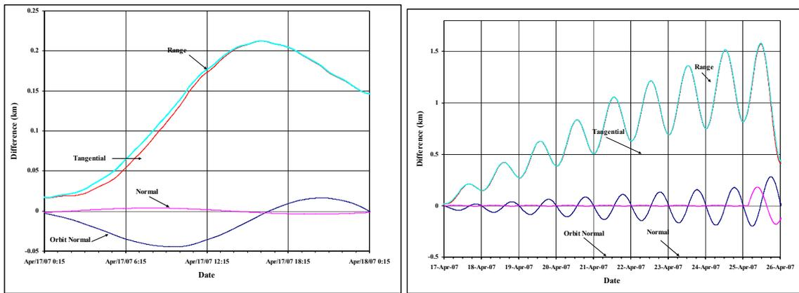
**Figure 17: GEO OD Ephemeris Comparisons:** Results are given for a GEO satellite after a 3 day OD of observational data. The difference after 1 day is about 200m.
