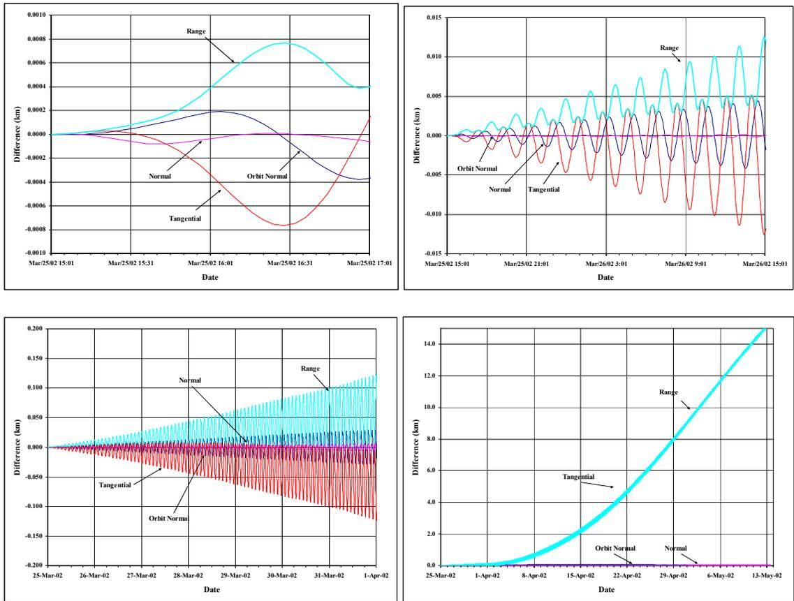
**Figure 8: Jason POE Ephemeris Comparisons:** Results are given for Jason at the four time intervals. The results are very similar to the ERS results.
