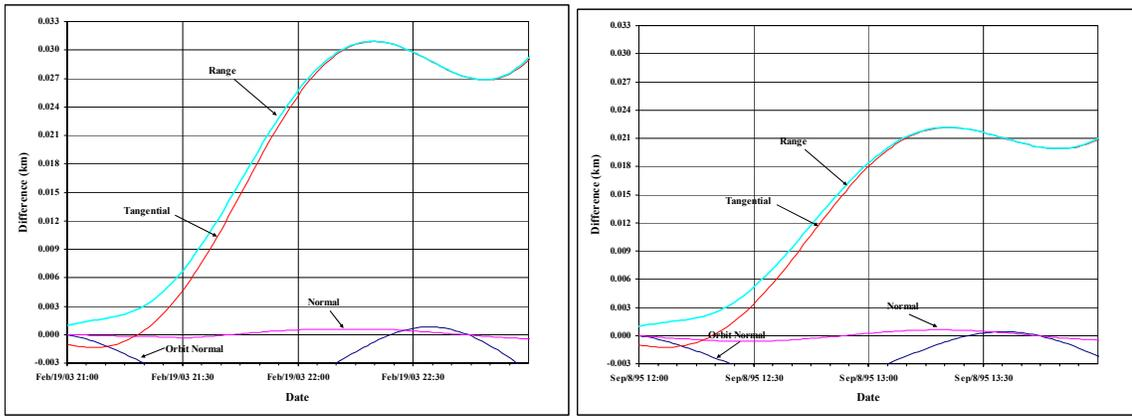
**Figure 11: POE Ephemeris Comparisons:** Results are given for ICESat (left) and ERS-2 (right). The similarity of the orbital altitudes produces very similar results. Notice the difference in the orbit normal component. In both cases, the dominant feature is the initial tangential displacement. The scales are the same between the two graphs.
