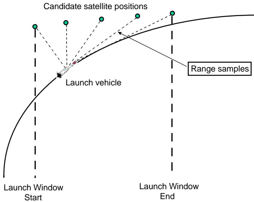
Figure 2. Locus of possible Earth-Centered Earth-Fixed positions for a candidate object considering the launch window
