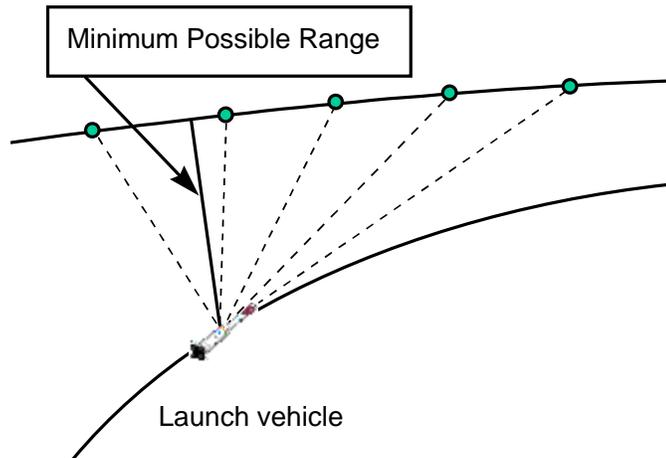
Figure 3. Minimum possible range at a specific time past time of launch
