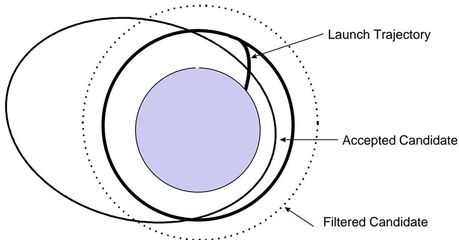
Figure 1. Application of the apogee/perigee filter
