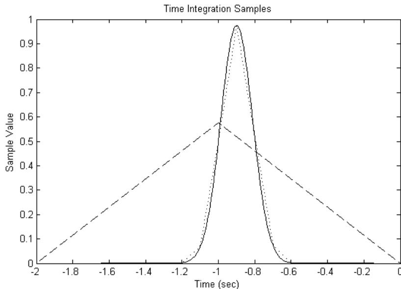
**Figure 2. The effect of step size selection on time integration for one sample point on the sphere. The dashed line shows samples at 1 sec; the dotted line at 0.1 sec; and the solid line at 0.01 sec.**
